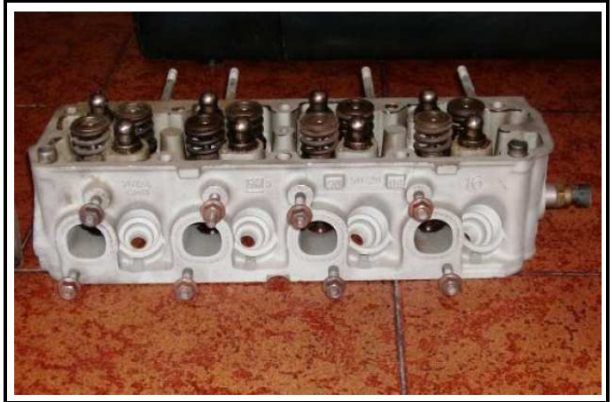
C8-6) Tapa desarmada vista lado salida escape Bare cylinderhead seen from exhaust side
