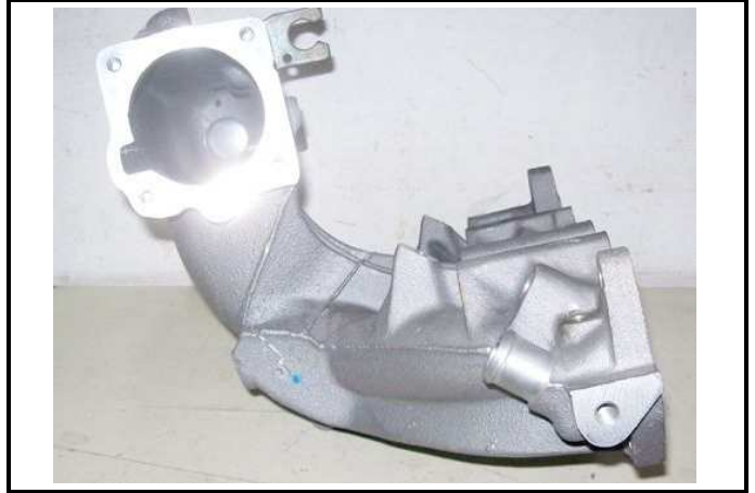
C11-2) Multiple de admision – desarmado Intake manifold - dismounted
