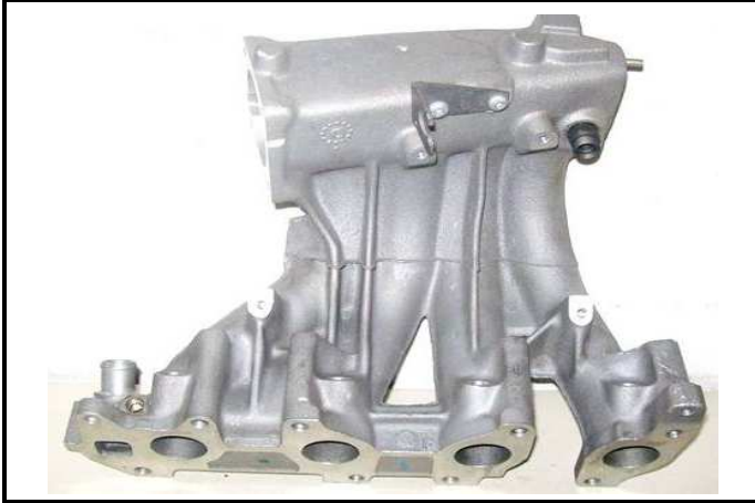
C11-1) Multiple de admision - desarmado Intake manifold - dismounted
