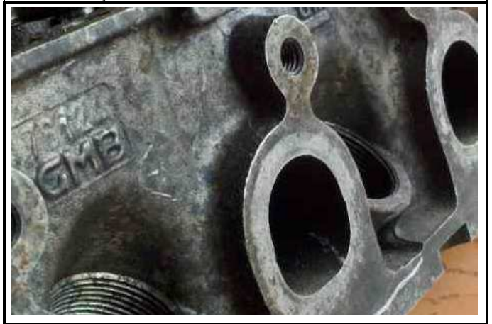
C8-8) Tapa desarmada vista lado salida escape Bare cylinderhead seen from exhaust side
